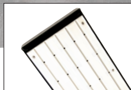
Storage tray with nylon plates acts as a seaming weight
