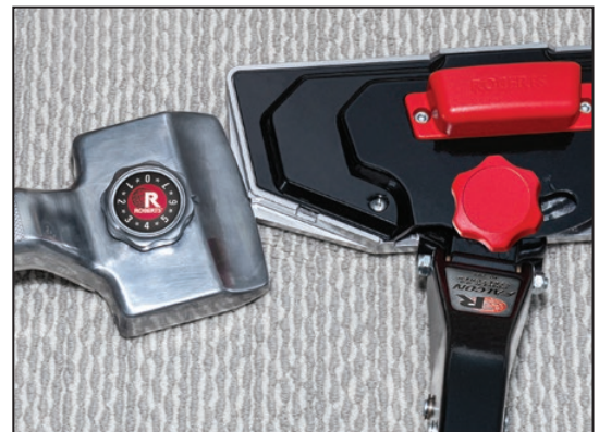
Low-profile head with side kicking platform for use with knee kicker
