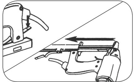
Insert a strip of fasteners into the magazine. Make sure the staple's crown is resting on the magazine.
