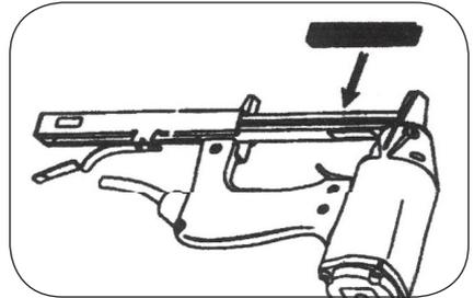
Push the magazine cover forward until the latch catches.
